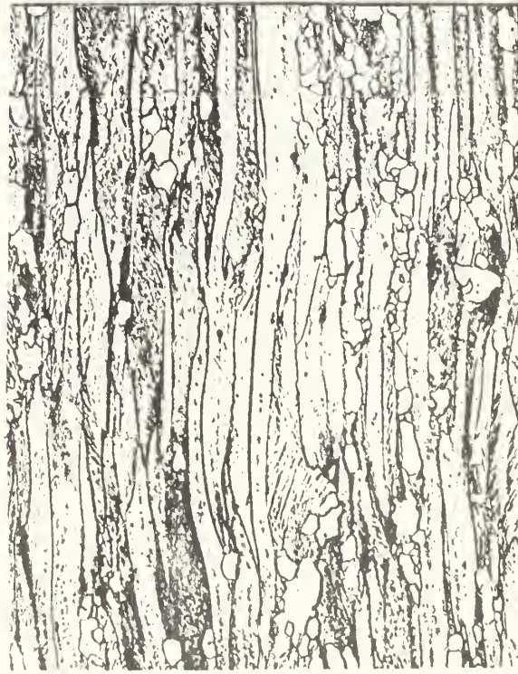
FIG.15 AT 482°C FOR 96 HOURS (ROCKWELL 30T 52.4) -150 X- FIG.16 AT 448.5°C FOR 1242 HOURS (ROCKWELL 30T 52.5)
